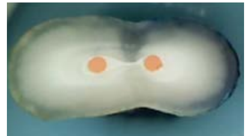
Optical microscope image of microleakage test (dye penetration test) ; No dye penetration
